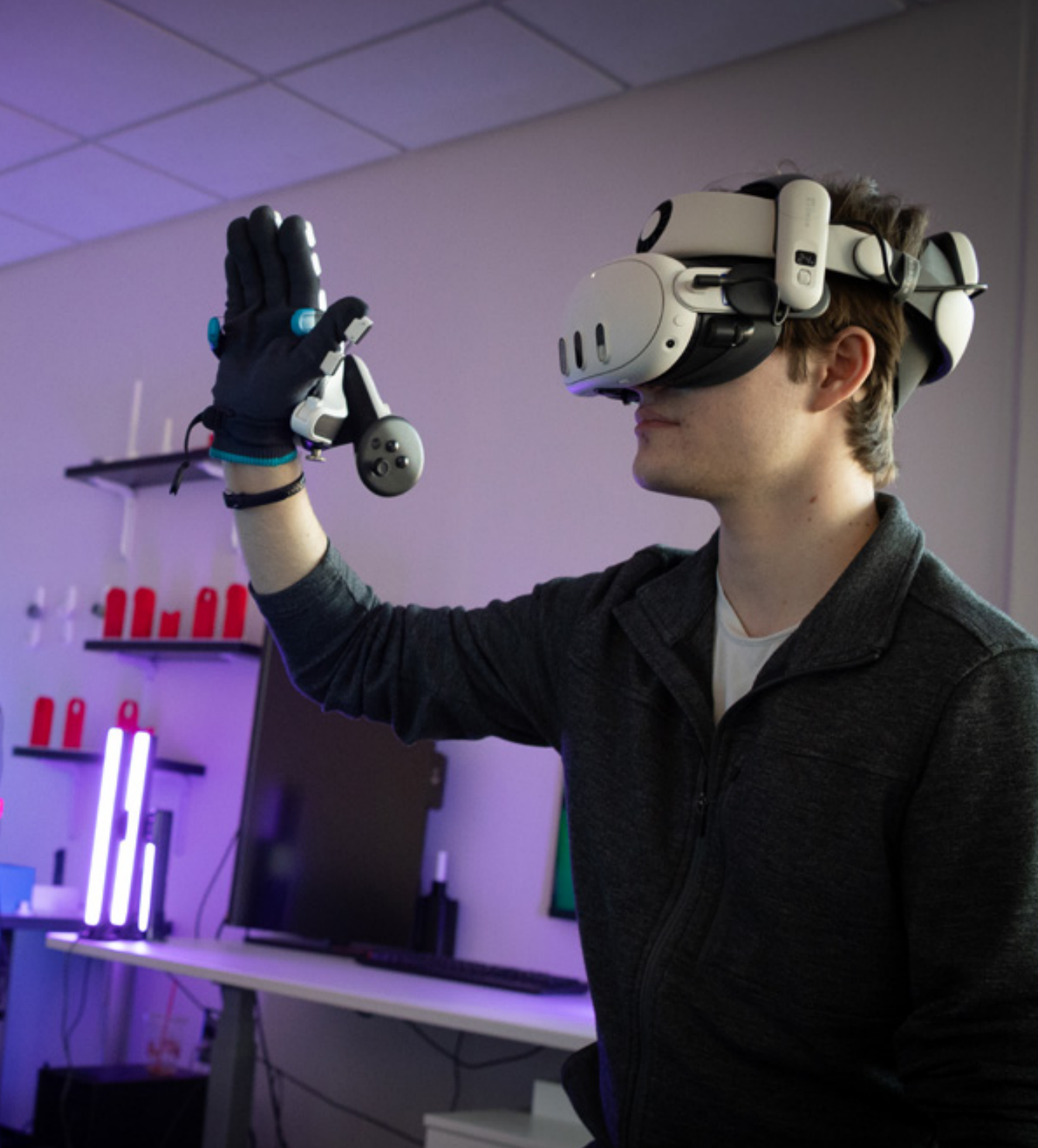
Left: Mechanical engineering Ph.D. student Austin Graves teleoperates a humanoid robot while wearing haptic gloves that provide tactile and kinesthetic feedback.
