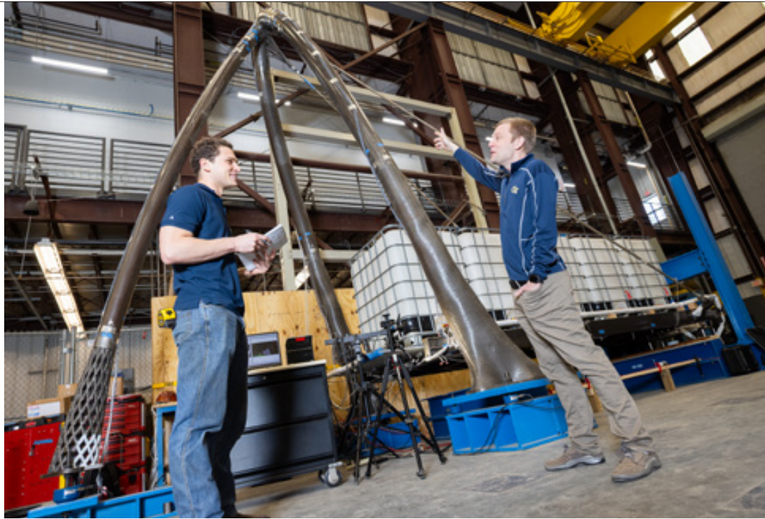
Above: Ryan Sherman (right) and Ph.D student Zachary de Haaff stand in front of a 17-foot-tall 3D printed modular section of a bridge that would be nearly 50 feet long. Sherman's team conducted load testing to demonstrate that the new additive manufacturing technology could meet performance demands.
